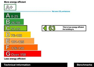
Main heating fuel: Grid Supplied Electricity Building environment: Air Conditioning Total useful floor area (m<sup>2</sup>): 124 Building complexity (NOS level): 3 Building emission rate (kgCO<sub>2</sub>/m<sup>2</sup>): 41.56
